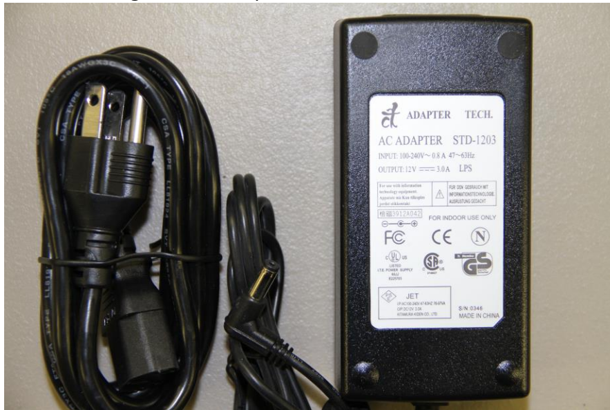
Power supply, 12 Volt DC regulated, 3 Amp
