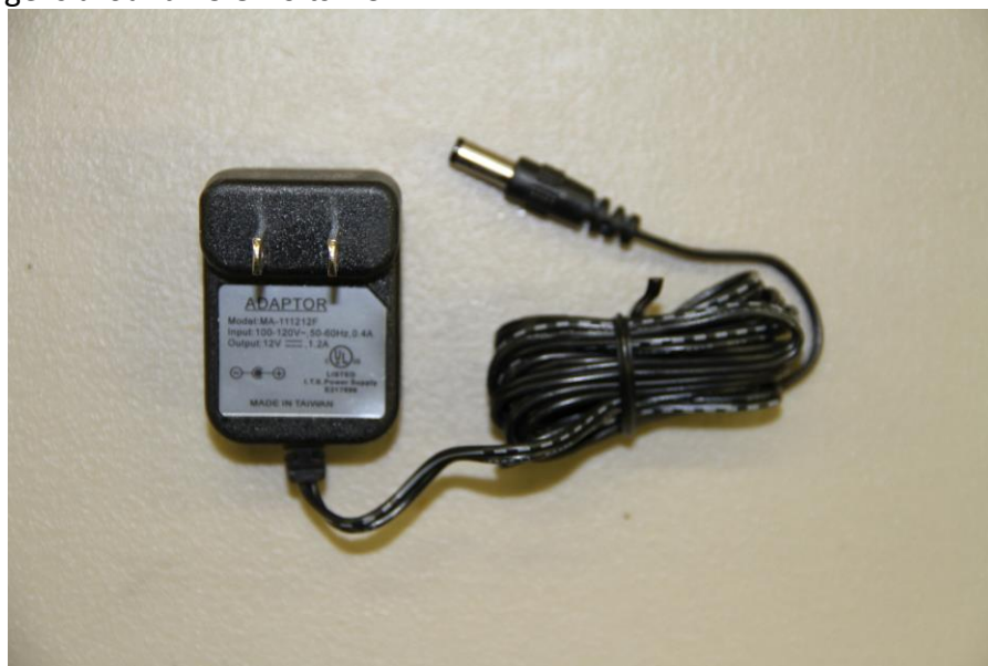
Power supply, 12 Volt DC UNREGULATED, 1.2 Amp No load voltage is around 13.8 Volts DC
