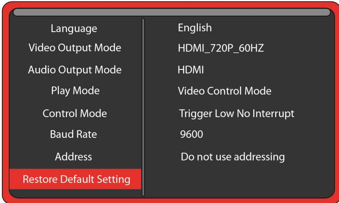
Select Restore Default Setting and press the green Enter key on the remote control. Then when the pop-up window appears, select “Yes” and press “Enter” to reset the Sprite® to the factory settings.
