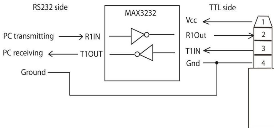
The MAX3232 can be powered from the Sprite®. Connect all Grounds together.
