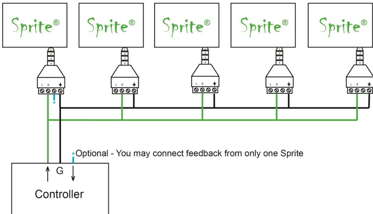
Limitations on the number of Sprites on the bus include length of wire, type of wire and baud rate. Low capacitance wire and lower baud rates will allow longer distances and / or more Sprites on the bus.
