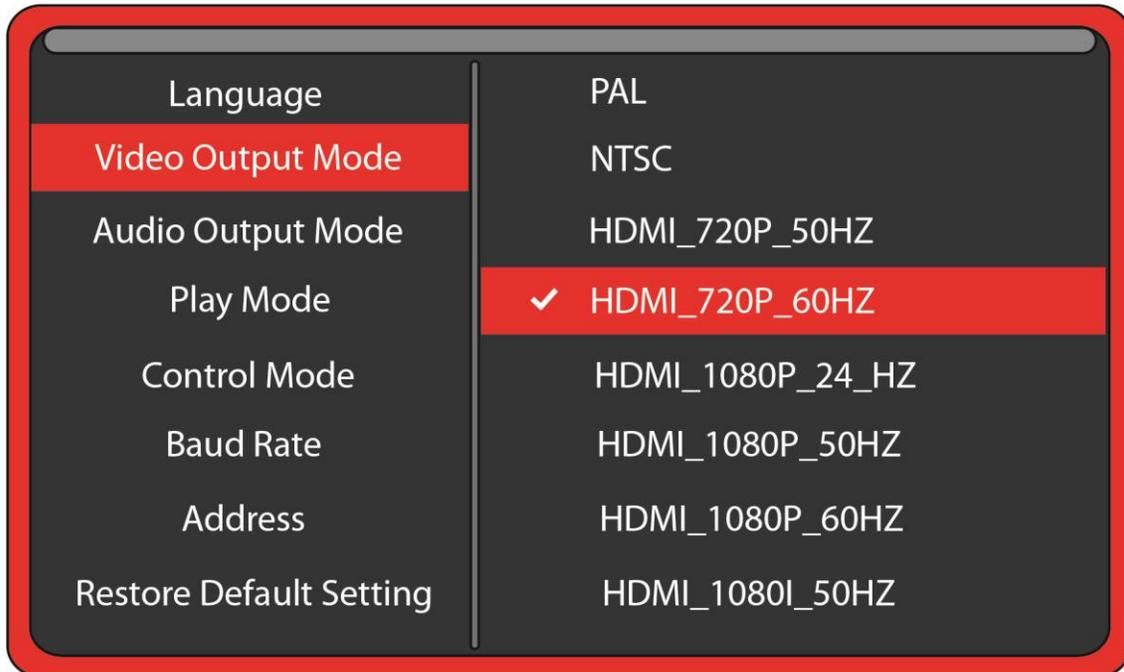
Select **NTSC** to use the Composite video output from the 3.5 mm yellow AV jack using the yellow RCA plug from the included A/V cable.
