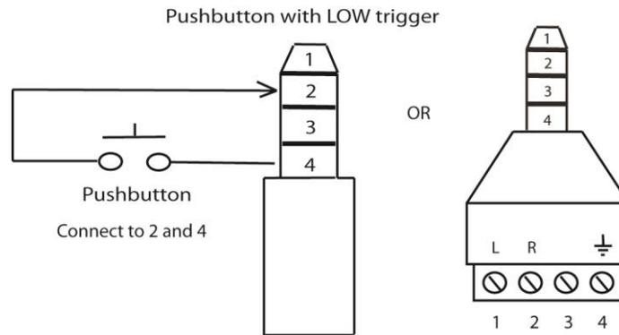
The Control Mode should be set to Trigger Low No Interrupt or Trigger Low with Interrupt.
