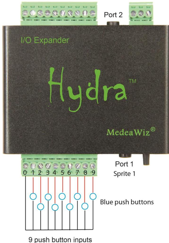
Each pushbutton should have 2 terminal connections.
